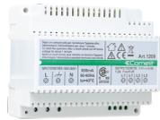
33 VDC power supply unit with overload and short circuit protection devices. It has two separate continuous outputs: one to power the external unit and electric lock, and the other to power the monitor. Input voltage 110-240 VAC. Dimensions: 106x62x89mm (6 DIN modules).
