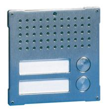
Module made using double 2.5 mm 316 stainless steel plate. For use with audio unit depending on the wiring system used. 2-button module. Dimensions 106x106x44 mm
