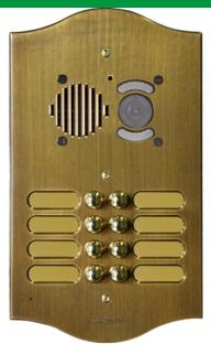
Door-entry monitor entrance panel with front plate in 3 mm thick bronze-finish watchmaking brass plate with PVD treatment. Complete with flush-mounted box and anti-intrusion screws. All entrance panels are fitted with bulb sockets (without bulb) for festoon bulbs with a diameter of 6.3 x 39. The entrance panel should be finished with an audio/video unit depending on the wiring system used. 24 buttons, 4 wires. Plate dimensions 340x362x3 mm. Box dimensions 320x296x55 mm. 3 bulb sockets
